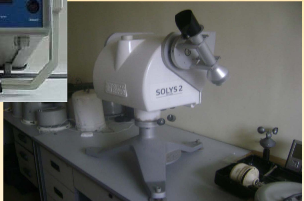
CHP1 pyrheliometer with Suntracker /Holland/
